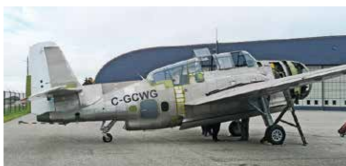
TBM-3E Avenger BuNo 53858/C-GCWG has been restored to represent a Royal Canadian Navy Avenger AS3, with the distinctive sloping rear canopy to aid visibility in the anti-submarine role. CWHM
