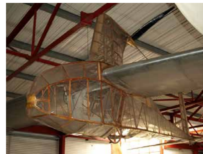
Now almost 60 years old, the SUMPAC human-powered aircraft hanging from the ceiling at Solent Sky. Note the large pylon for the pusher propeller.
