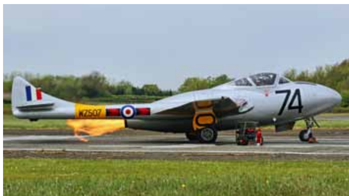
A spectacular 'wet start' by the Vampire T11 on the second day of the fly-in
