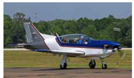
Civilian-owned P & W PT-6-powered early prototype of the Polish PZL-130T Turbo Orlik
