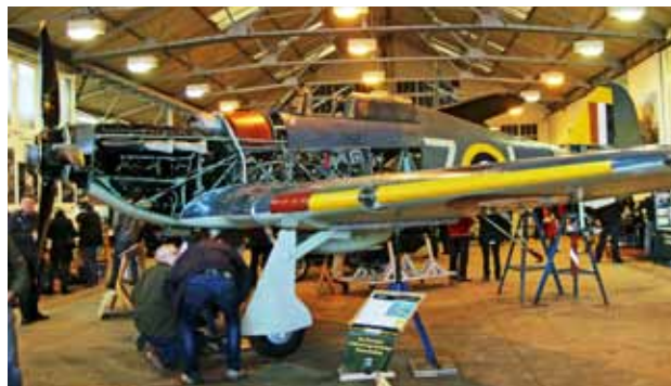
Undercarriage retraction tests were demonstrated on Sea Hurricane Z7015, mounted on jacks and stripped of its main access panels
